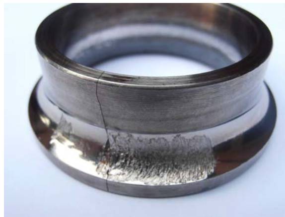
Fig. 1.2: Axial cracking on bearing ring.
