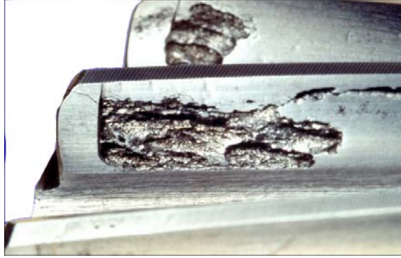
Fig. 1.1: Fatigue occurrence on a Roller bearing.
